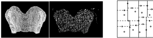
Fig. 4. Left: 3D model from CT and from structured light Right: 2D kd-tree
