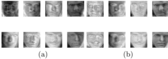
Fig. 2. Principal components vs. canonical vectors. (a) The first 4 principal components computed from the two image sets shown in Figure 1. The principal components of the different image sets (see each column) show significantly different variations even for the same objects. (b) The first 4 canonical vectors of the two image sets. Every pair of canonical vectors (each column) well captures the common modes (views and illuminations) of the two sets, i.e. the pairwise canonical vectors are almost similar.
