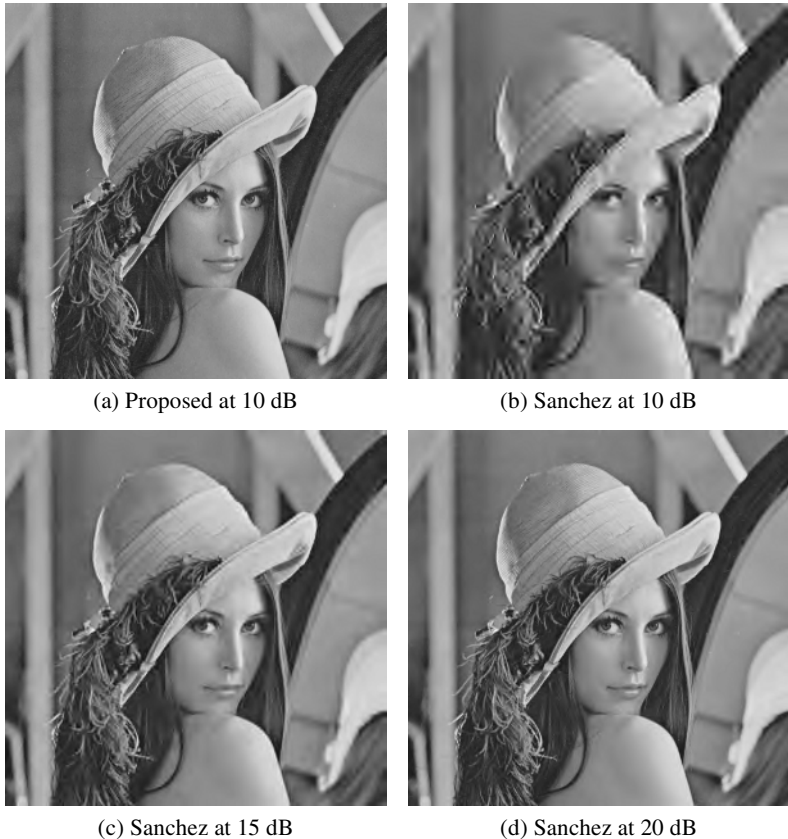
Fig. 6. Visual results for ‘Lena’ image at R_T = 4.41 bpp. (a) Reconstructed after transmission via proposed scheme at E_b/N_0 = 10 dB (PSNR = 42.59 dB), (b) Sanchez et al. at 10 dB (PSNR = 26.88 dB), (c) Sanchez et al. at 15 dB (PSNR = 31.59 dB), and (d) Sanchez et al. at 20 dB (PSNR = 36.27 dB).
