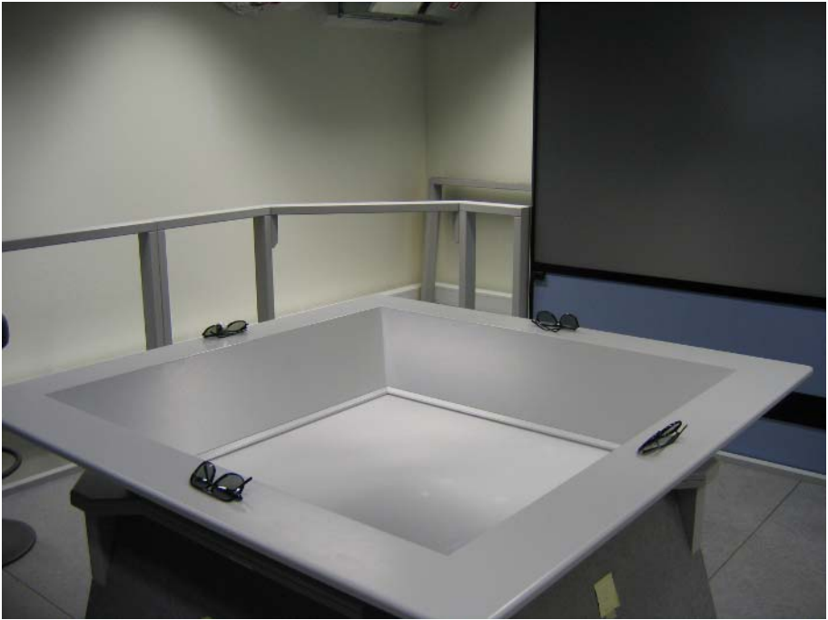
Fig. 1. The display used in the experiment can provide four independent stereoscopic views
