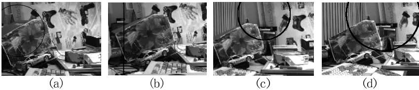
Fig. 5. The zero-boundaries determined by estimated FOEs. (a) Camera A, Motion 1, \mathbf{s}=[0 \ 0 \ 1] ; (b) Camera A, Motion 2, \mathbf{s}=[1 \ 0 \ 0] ; (c) Camera B, Motion 1, \mathbf{s}=[0 \ 0 \ 1] ; (d) Camera B, Motion 2, \mathbf{s}=[0 \ 0 \ 1] .
