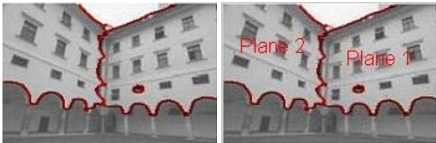
Fig. 3. The final segmented components of the left image using the normalized cut algorithm ( left ) and the detected planes from the Minorite Monastery data ( right )
