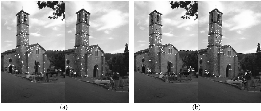
Fig. 1. Correspondences of the Valbonne church image pair. (a) Using the SIFT. (b) Using the Harris corner detector and correlation-based matching.
