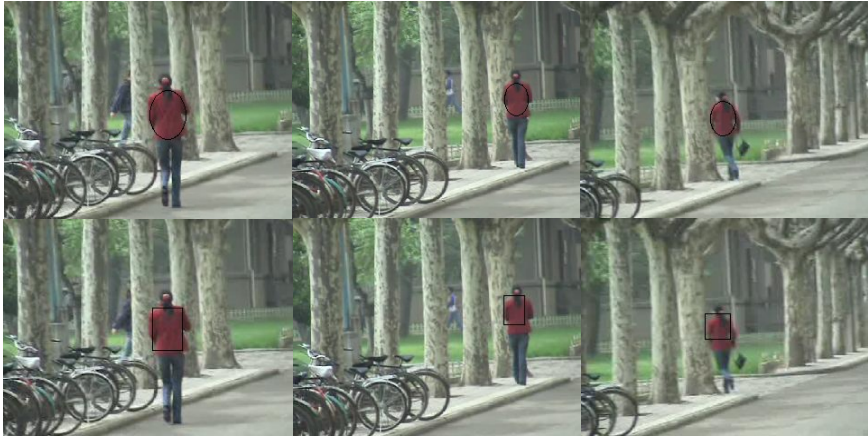
Fig. 5. Tracking results of a pedestrian. Upper row: Results based on our method. Lower row: Results of the bandwidth mean shift tracker. Only the 3 rd , 254 th and 341 st frames are shown.
